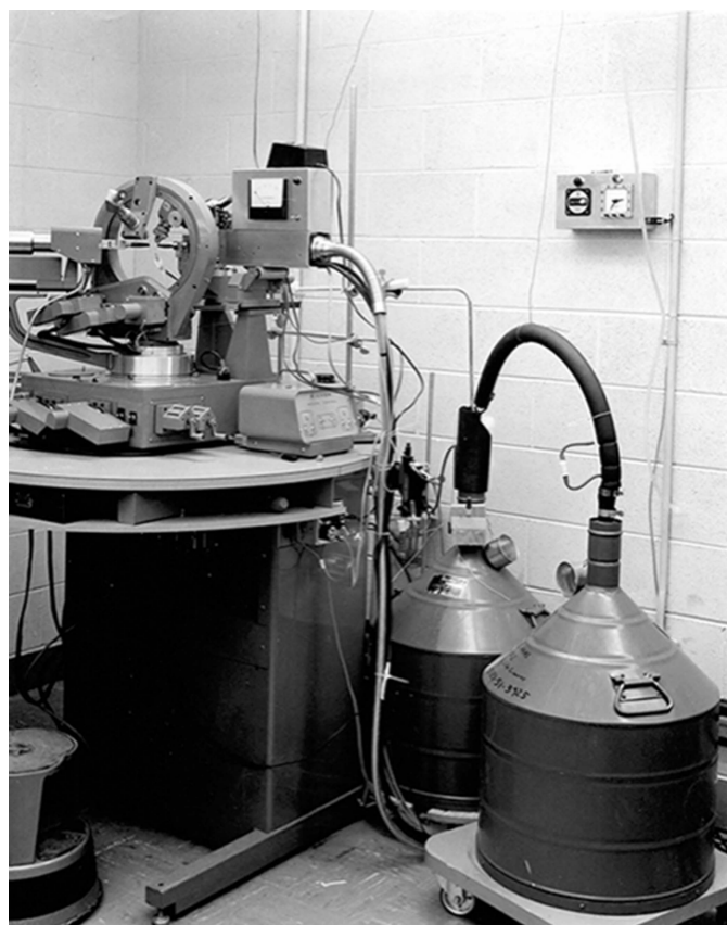
Figure 6 The cryo-cooling apparatus used at Purdue University in 1968 for lactate dehydrogenase data collection (Haas & Rossmann, 1970). The Dewar on the left is as shown in Fig. 4, while the Dewar on the right is transport for refilling. (Photograph by D. Haas.)
