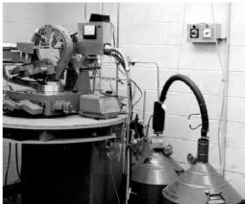
*Freezing apparatus in the Rossmann lab for collecting the first data from frozen LDH crystals.*
